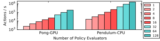
Figure 7. Policy evaluation throughput scales nearly linearly from 1 to 128 cores. PongNoFrameskip-v4 on GPU scales from 2.4k to \sim 200 k actions/s, and Pendulum-v0 on CPU from 15k to 1.5M actions/s. We use a single p3.16x1 AWS instance to evaluate from 1-16 cores, and a cluster of four p3.16x1 instances from 32-128 cores, spreading actors evenly across the cluster. Evaluators compute actions for 64 agents at a time, and share the GPUs on the machine.
